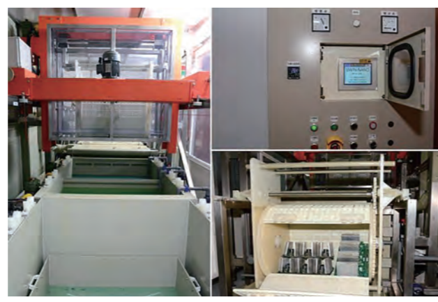
▲Barrel One機台單日可處理多達兩千片廢PCB。uwinnano.com
